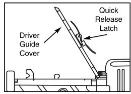
Figure 5. Removing guide cover.
